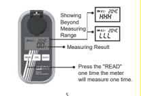
If press the "Read" button for 2 seconds, the instrument would make the automatic measurement upon programmed times (default 15times), the final value is the average of 15 times' measurements. After measurements. the multi-functions display area would return back to scale showing status.
