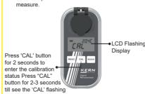
Press "CAL" button once again during the 'CAL' flashing to start to calibrate. When the calibration is completed showing as following. If no any operations for 10seconds the instrument would return back to booting status.
