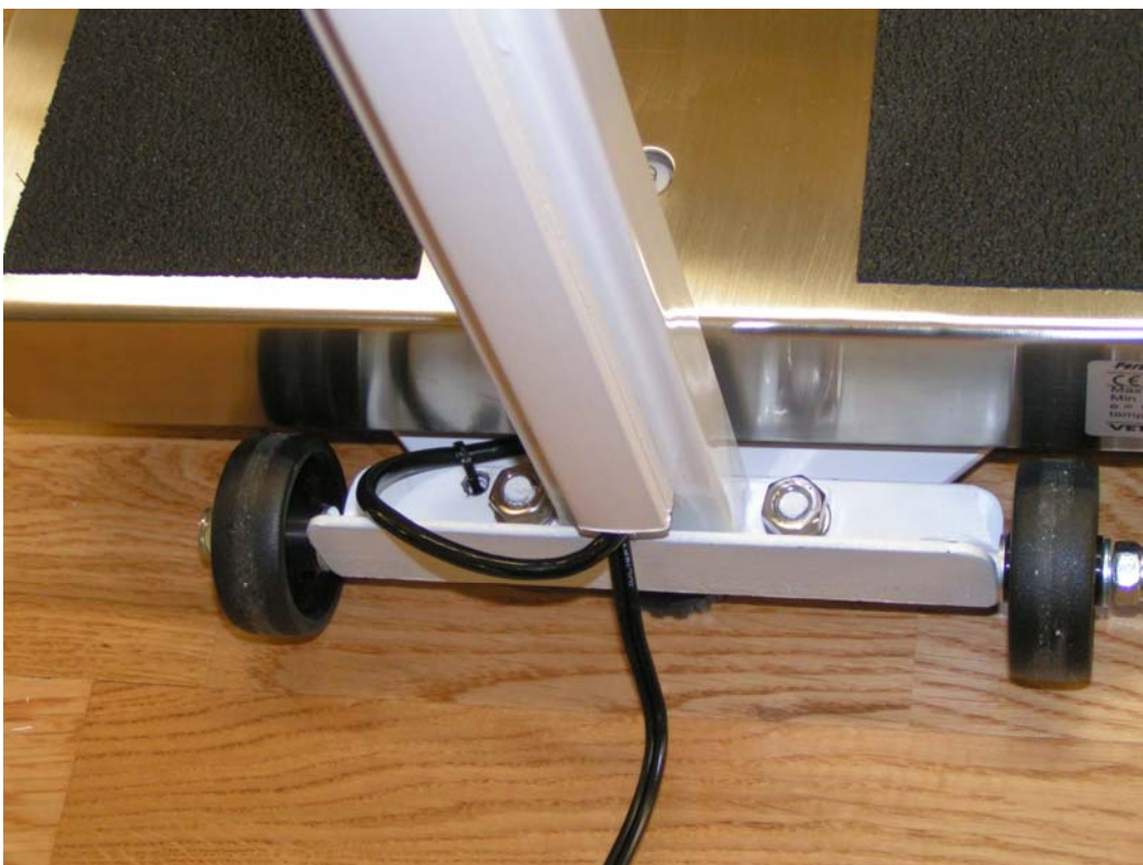
This is how the wheels are assembled together with the column (option).
