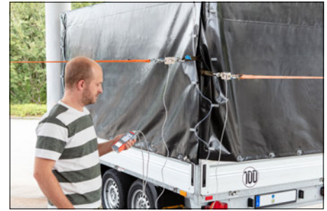
Measurement of forces in different tensile or compressive directions possible with only one measuring device
