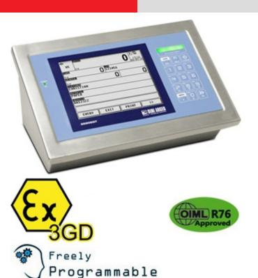
Weight indicator with a big touch screen display, suitable for advanced industrial applications in ATEX areas classified at risk of explosion with protection methods according to ATEX II 3G Ex nR IIC T6 Gc X ATEX II 3D Ex tc IIIC T135°C Dc IP68 X. Fitted with programmable inputs and outputs, 3 serial ports, completely configurable printouts, and integrated alibi memory. CE-M approvable (OIML R-76 / EN 45501).
