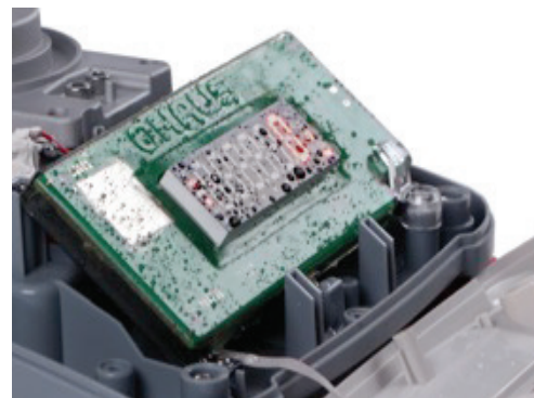
Inside PCBA Silicon Glue Sealing
