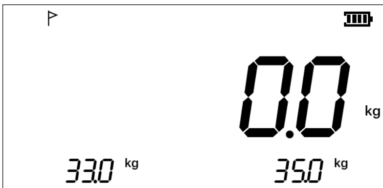
Figure 4-5 Upper/Lower Limit Alarm Function
