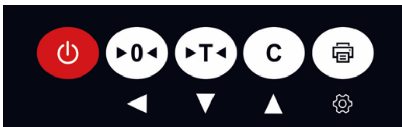
Figure 4-2 Instrument Panel Navigation Keys
