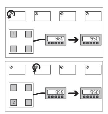
Calibrate the scale with a sample weight and verify again that all the corners display the same weight.
