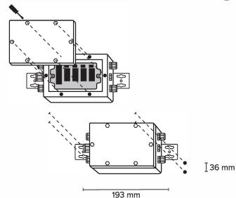
To ensure the IP rating use only cable glands and O-rings from Dini Argeo; Use only in environments not harmful to stainless steel and silicone
