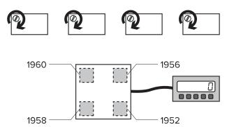
Place a weight on each load cell and identify which one of them displays the greatest weight. Adjust the trimmers on the board counterclockwise until all load cells show the same weight, as in the following example.
