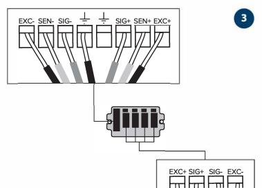
If the load cells have 6 wires, cut SEN+ e SEN- wires or connect together SEN+ with EXC+ and SEN- with EXC-.
