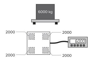
Screw all trimmers clockwise and calibrate the scale.
