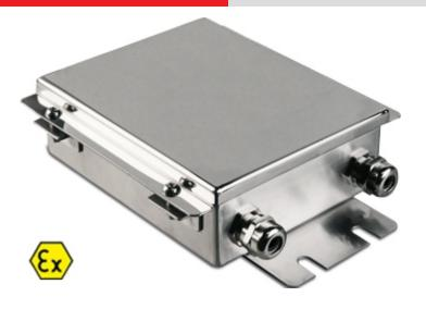
Stainless steel junction box with IP66 protection from water and dust, and fitted with an intrinsically safe electronic board for junction and equalisation of load cells. Terminal boards with screws for easing th connection of the load cells and signal adjustment trimmer, for an accurate and reliable equalisation.
