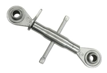
Galvanized stay rod, useful to limit the movements of the weighed structure without affecting the weighing results. Fitted with two ball-and-socket joints (overall lenght adjustable from 260 to 350mm).
