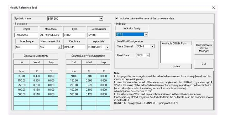
This page stores all the data related to the Reference Tools that can be used to perform the calibration. For correct operation it is necessary to correctly fill all the following fields that can be easily recovered by an ACCREDIA (or equivalent) calibration certificate.
