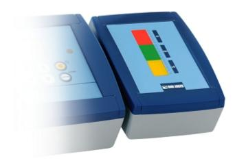
Option Box with 3-way control light with programmable acoustic signal, bar graph controller, attachable to DFW and 3590 series' indicators. The control light allows to independently manage the 3 LUMINOUS AREAS and the BUZZER, using the TTL logic.
