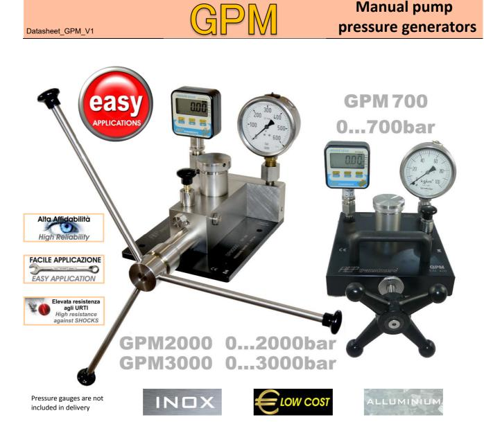
The **GPM** manual pressure generators are a system created to solve the problems of calibration and checking of dial manometers, transducers, pressure transmitters and pressure switches with a first line sample carrying ACCREDIA certification.
