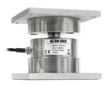
Thanks to the ELGO modular kit, it is possible to quickly install CP/CPX compression <u>load cells</u>, up to 12.500kg, for weighing of silos, tanks, or different kinds of structures, containing installation costs. Built in STAINLESS steel and extremely simple to clean, ELGO is ideal for weighing in environments which are hostile, or that have high hygiene requirements. ATEX certification II 2GD c IIC T6 85°C.
