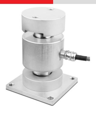
Analogue version of compression load cells, 4000 divisions, ideal for CE-M approved weighbridges, tanks, silos, etc. STAINLESS STEEL execution, with IP68 protection, fitted with "anti rat" shielded cable.
