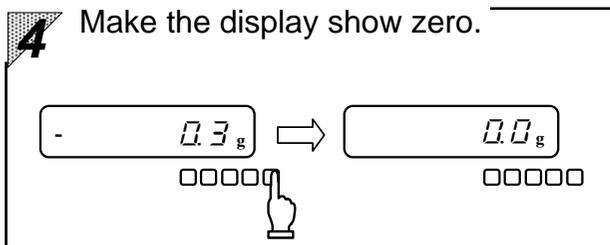
If the display readout does not become zero, press the
