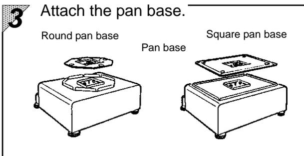
Set the pan base with its screw hole aligned to the projection on the main body and tighten the screw with a screwdriver or an appropriate coin.
