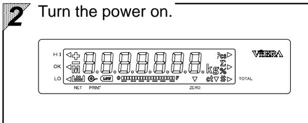
At this time, check that no LEDs nor LED segments stay out. After a few seconds, zero is displayed in the weight display.
