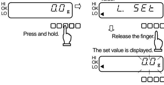
Press and hold the
