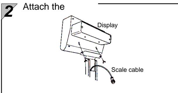
Pass the scale cable in the pole and attach the display to the pole.
