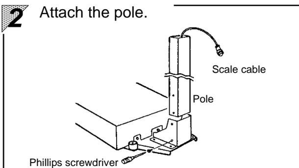
Pass the scale cable under the pole (from the wider side of the fitting hole). Next, attach the pole to the pole base.
