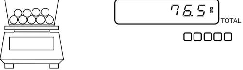
When additional samples are placed in the container, the weight of only the added samples is displayed.
