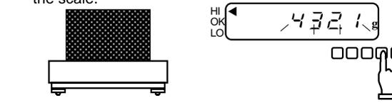
Place the sample for the upper limit value on the scale and press the
