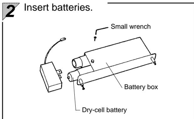
Remove the battery box cover with the small wrench in the accessory kit.
