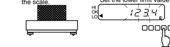
Place the sample for the lower limit value on the scale and press the
