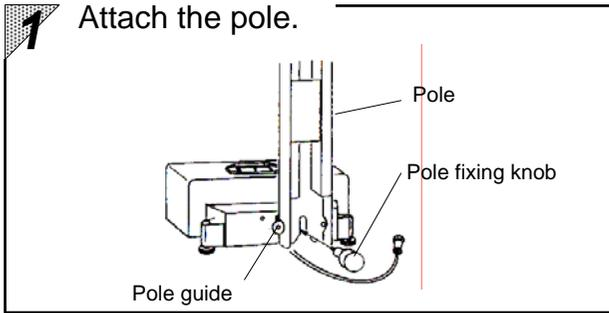
Install the accessory pole to the rear guide with the pole knob.
