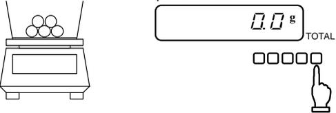
When additional samples are placed in the container, press the
