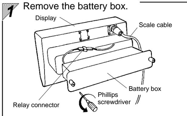
Loosen the screw in the rear of the display and the battery box can be removed.
