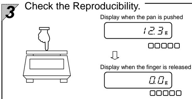
Push the pan slightly using your finger to check that the display readout changes. Also check that zero is indicated in the display after the finger is released.
