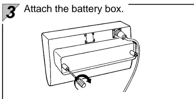
Connect the relay connector of the battery box and install it on the display.
