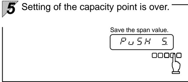
When calibration of capacity point is over, "PUSH 5." is displayed. Press the
