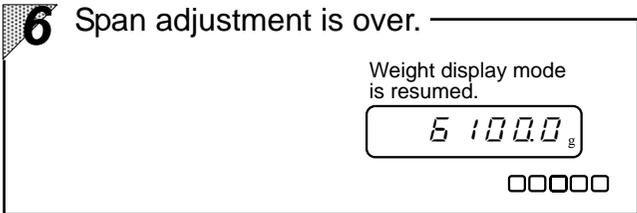
The weight display mode is resumed and span adjustment is completed.
