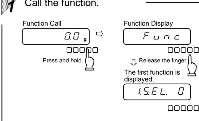
Press and hold the
