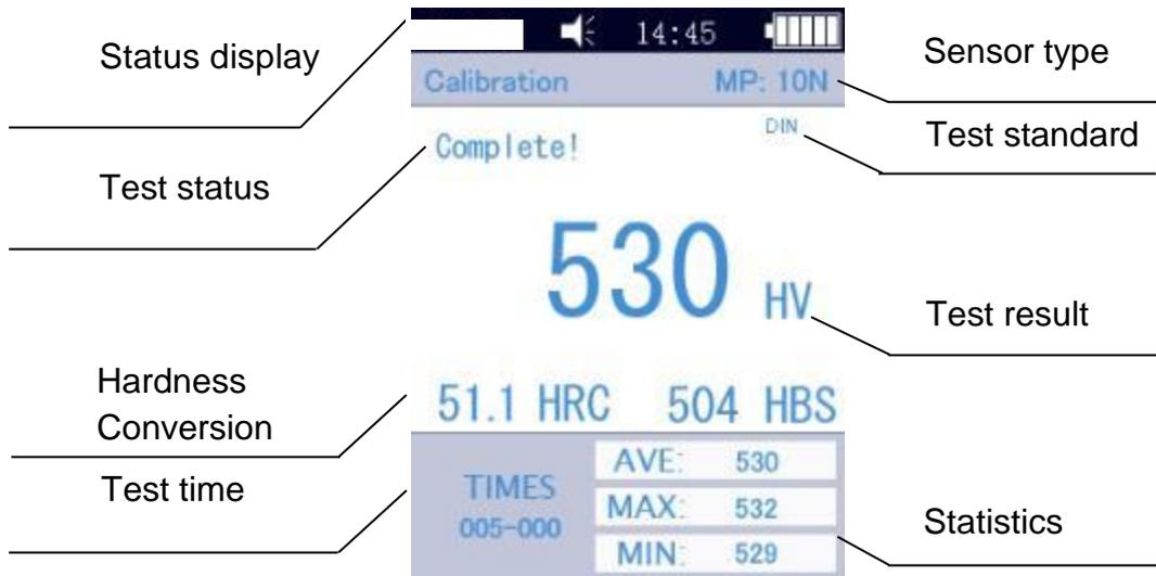
The menu masks contain status display, model info, calibration data, test display, result list and info list for test results as shown in Fig. 6-3.
