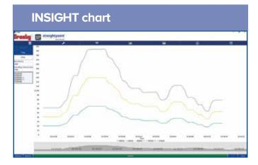
INSIGHT software, supplied with an SW-D USB wireless dongle, allows connection of up to 126 Straightpoint wireless load cells simultaneously onto any Windows tablet or laptop.
